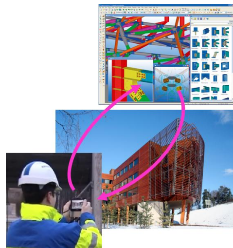
Figure 1. Mixed reality interaction cycle: mobile view of construction site augmented with BIM (arrow down), and feedback from mobile device back to BIM (arrow up).
